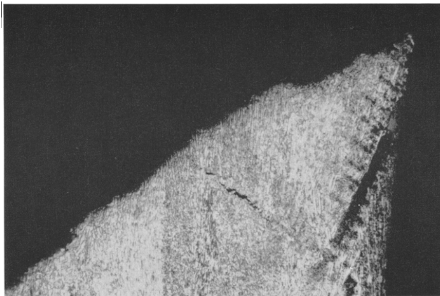
Figure 4 The composite with metal dendrites. Longitudinal section in the neighbourhood of the fracture surface for a sample containing 2.8 wt % C tested at 900°C in air (magnification \times 200 ).
